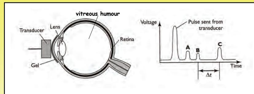
The simplified diagram above shows an A-scan of the human eye. The reflected pulses **A** and **B** are from the front and back of the eye lens. Pulse **C** is produced by the ultrasound reflection from the retina.
