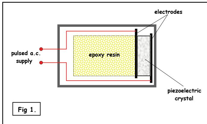
The piezoelectric crystal is backed by a slab of epoxy resin, and the power supply to the electrodes either side of the crystal is pulsed.
