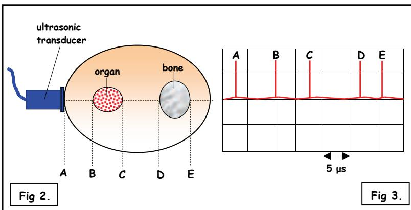
Fig 2. shows a cross-section through a part of the body. Ultrasound is pulsed through the centre of the section so that it passes first through an organ and then through a bone.
